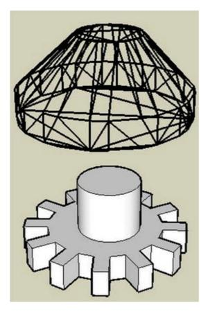
You can see that the convex hull made a shape similar to the gear above, but if you tried to make it "work" with another gear, it wouldn't. So how do you fix it? Let's look at a similar shape that I had a problem with. I encountered this situation when using "CONVEX HULL" to make an upside-down arch:
