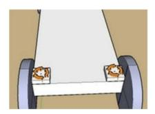
Now we'll need to use the UI to set the steering servos to behave as needed. Set each servo's min and max to -45 and 45 to limit their swing. Also set their controller name the same (I'm using "steering") so they'll work together.
