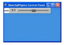
By default, the slider bar is at 0.5 (or at rest). By sliding it either left or right, we can make the hinge spin in either direction. The further you slide it, the faster it will spin in that direction.
