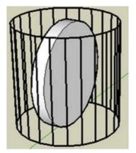
This cylinder object was set to "cylinder", but by using the DEBUG option, you can see the black wireframe shows SP thinks it is actually on it's side. If any other object interacts with this cylinder, it will hit the black wireframe, NOT the actual grouped shape!
