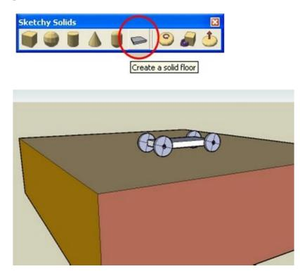
RUN the animation and you should be able to drag the car around the ground plane with the wheels spinning as it moves.
