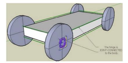
By doing this, we have given the hinge a "parent" object. (The body) It is now connected to the body, and it will spin in relation to the body. And since our wheel is grouped with the hinge, it will spin as the hinge does.
