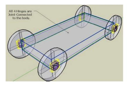
It's now time to test our car. If we RUN the animation now, the entire car would fall into space as one object. So let's make a ground plane for the car to rest on. You can either make a ground plane yourself and set it to "STATIC MESH" or you can use the auto-shape (SOLID FLOOR) to make the plane in one click.
